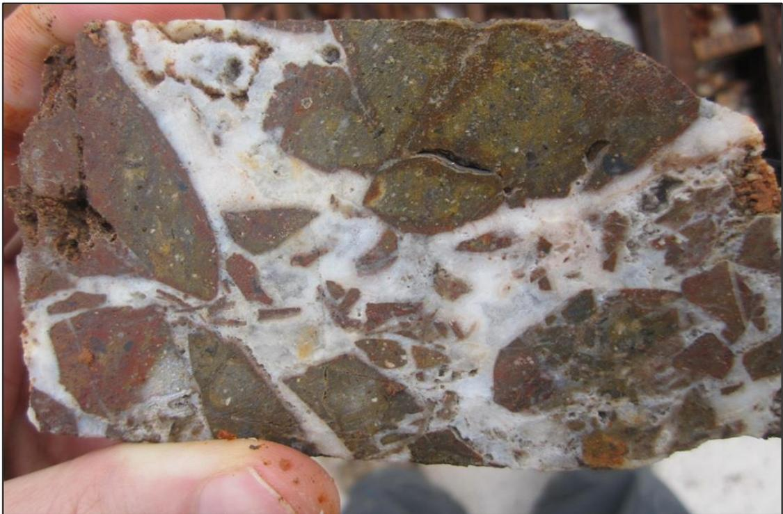
**Figure 7-7: Type 2 Gold Mineralised Breccia of the La India-California vein (Source: Condor, June 2012)**
