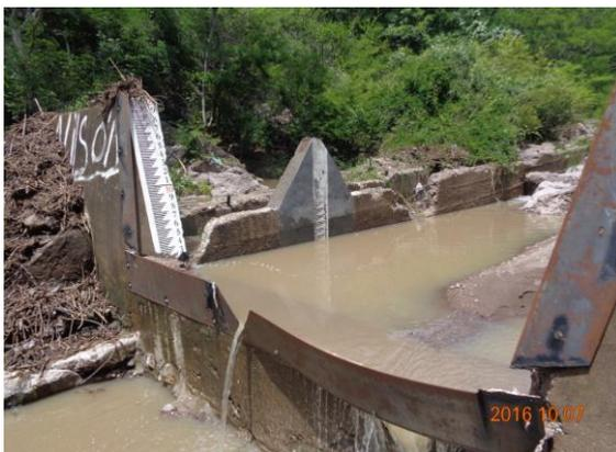
**Figure 3-1: La Simona v-notch weir failure on 07 October 2016**
