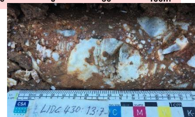
Fault brecciated quartz vein (mod-high Au grade).
