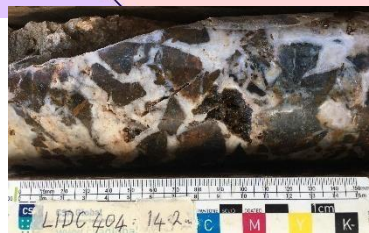
Footwall quartz breccia (low-moderate Au grade).
