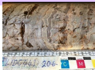
Banded chalcedonic quartz vein (mod-high Au grade).
