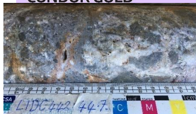
Multi-stage quartz veining (high Au grade).
